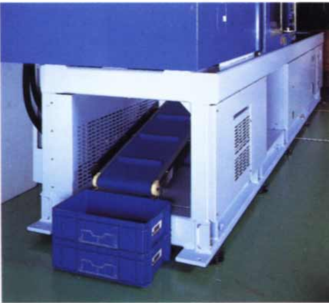
● Fitting of a molded parts conveyer (Conveyor is optional)
